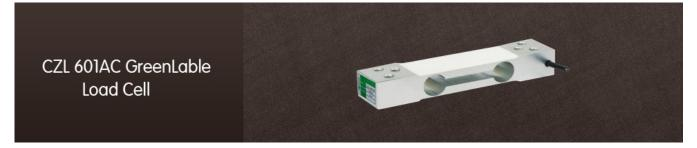
Model CZL 601AC (Table Top- Greenlable) is strain gauge based LoadCell constructed from Aluminum Alloy for high Accuracy. It is mainly used in check weighing. Suitable for Platter size upto 400mm X 400mm.
