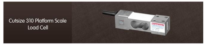
Cutsize 310 is a straingage based Single point parallel beam, low profile Platform steel loadcell. They are economical and have good performance characteristics suitable for small platform scales. They are made from high tool steel alloy with Electroless nickle platting for protecting loadcells from jerk loads & corossion. Its high tool steel construction make loadcell very Rugged to absorb shock loads.
